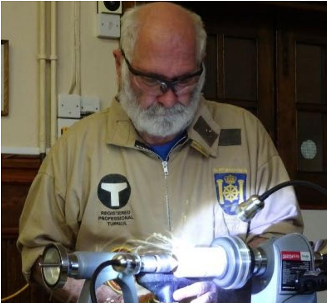
Starting with the square section spindle (Castello Boxwood) turned to round, designate the lid section as being closest to the chuck as it is easier to cut the male thread in the base. (I assume that this would not necessarily be required if a spigot had been created on each end of the spindle in the first place) Having cut off the lid section leaving a "witness mark" for aligning the lid and base screw threads, hollow out the lid and then cut the female thread.
