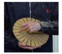
Having marked the lines it was then possible to hand draw the curved lines which were then carved out using a Proxxon mini-grinder ...
