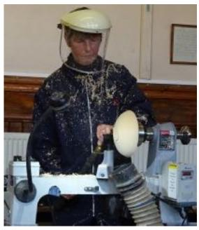
Starting with a pre-prepared ash blank Liz turned the base of the bowl using the standard method of truing up the outside and front faces, creating a spigot to fit the C Jaws, and then shaping the underside of the bowl using a series of push and pull cuts with a bowl gouge, finally sanding to 320 grit followed by 50/50 cellulose sanding sealer.
