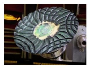
The inner bowl was then carefully turned with a bowl gouge and sealed, ensuring the sealer did not extend over into the rim as it would possibly remove some of colour.
